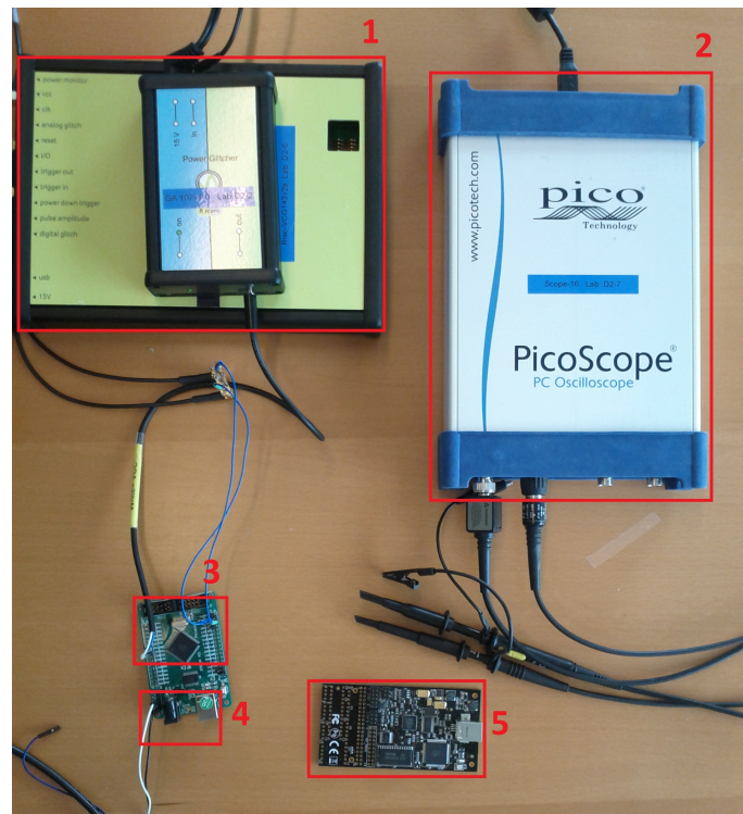
Figure 4.2: The test setup. 1: Voltage glitcher 2: Oscilloscope 3: Target IC 4: Serial connection 5: JTAG programmer
